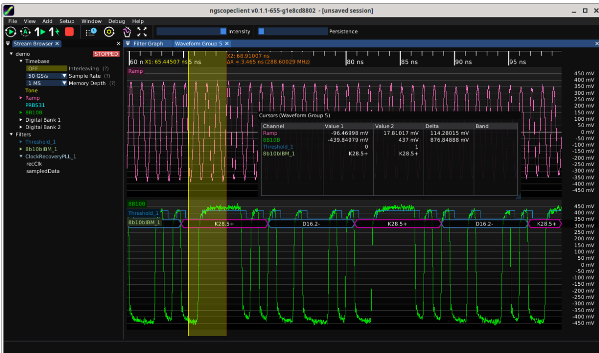
Figure 9.7: Double vertical cursor
