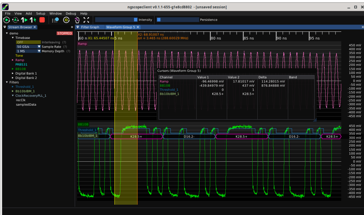
Figure 9.7: Double vertical cursor
