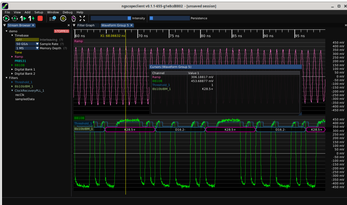
Figure 9.6: Single vertical cursor
