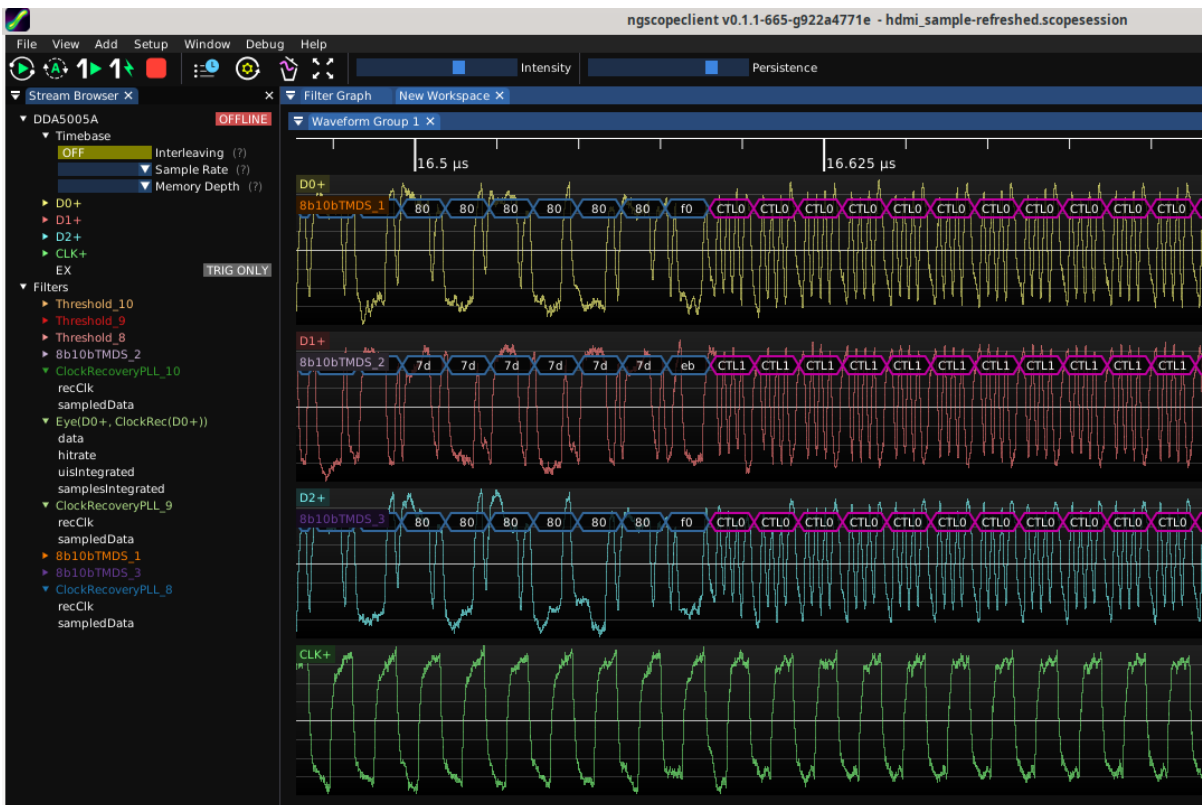
Figure 26.9: Example TMDS decode
