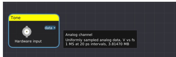
Figure 12.4: Tooltip on output port showing the available data
