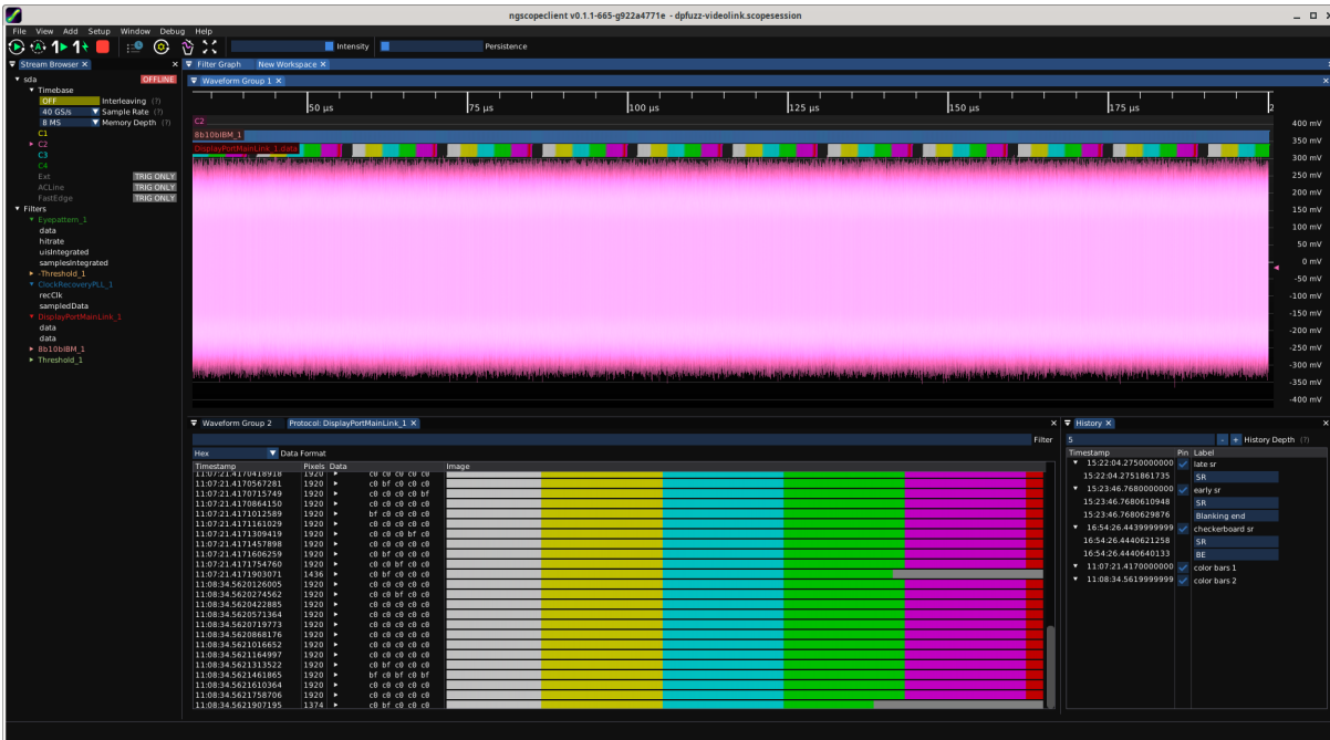
Figure 26.78: Example of decoding DisplayPort main channel
