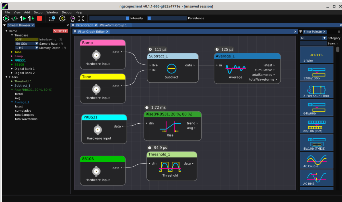
Figure 12.1: Filter graph editor showing instrument channels and several processing blocks
