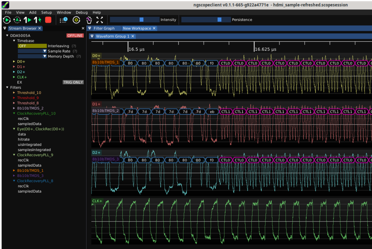
Figure 26.88: Example of decoding a DVI signal
