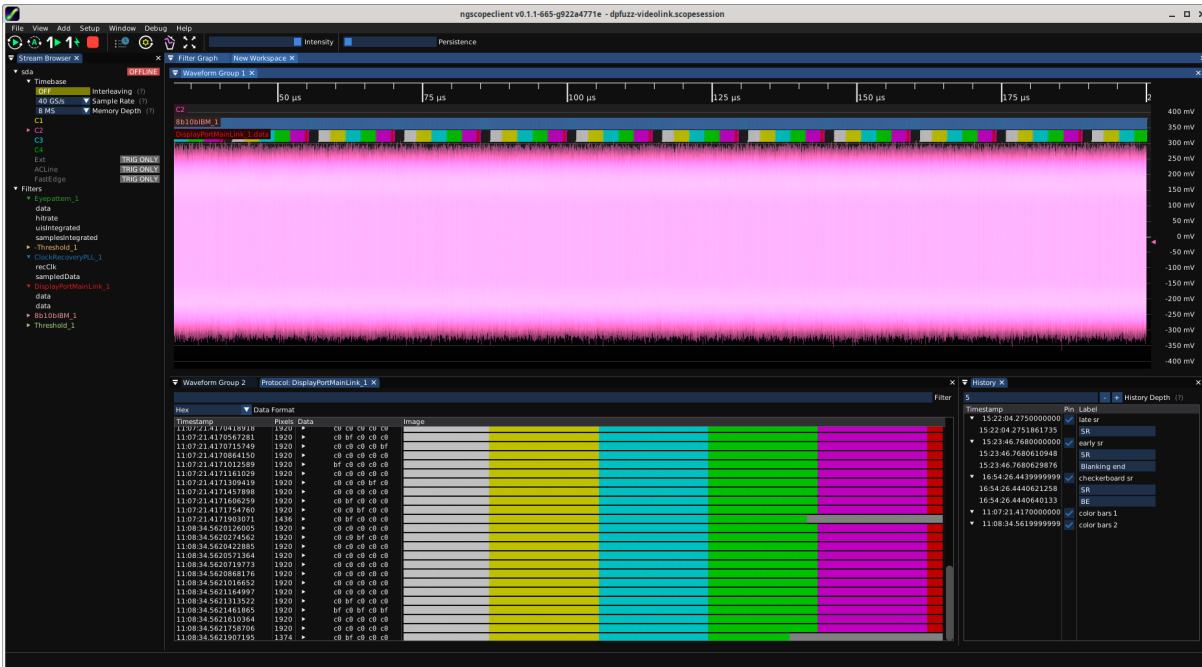
Figure 26.78: Example of decoding DisplayPort main channel
