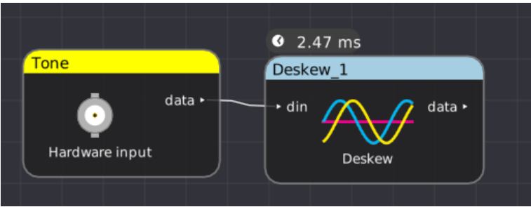
Figure 26.69: Example filter graph showing usage of deskew filter
