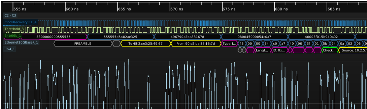
Figure 26.5: Example 64b/66b decode
