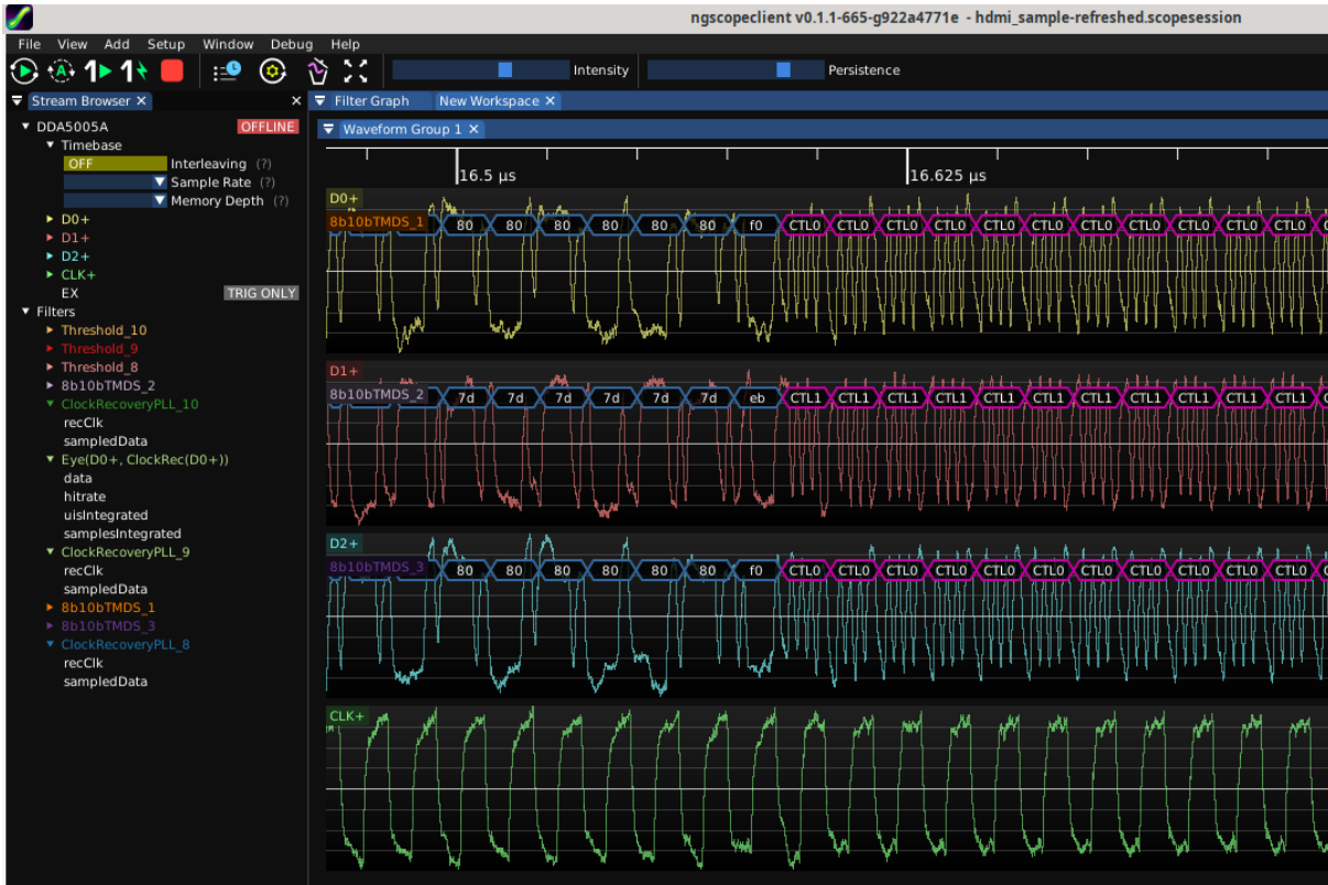
Figure 26.88: Example of decoding a DVI signal
