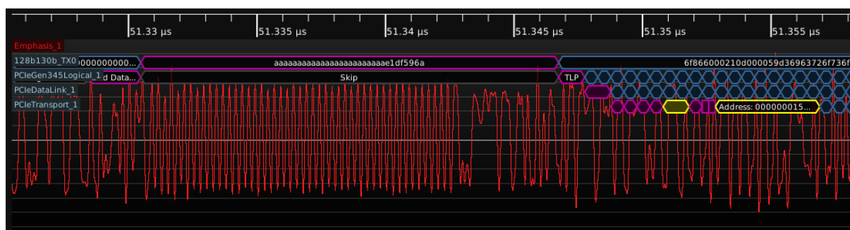
Figure 26.3: Example 128b/130b decode
