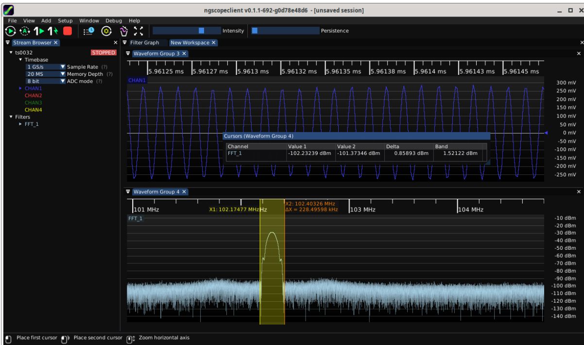
Figure 26.139: Example showing FFT of a modulated signal and using cursors to measure total in-band power
