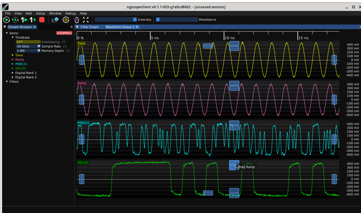
Figure 8.2: Overlays showing drag-and-drop locations for splitting waveform groups
