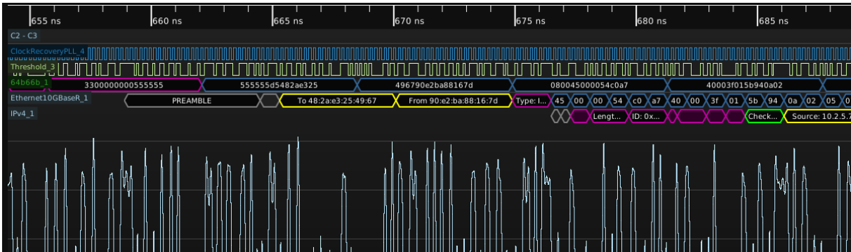
Figure 26.5: Example 64b/66b decode
