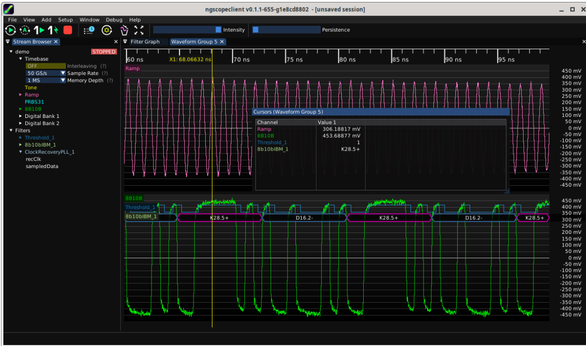
Figure 9.6: Single vertical cursor
