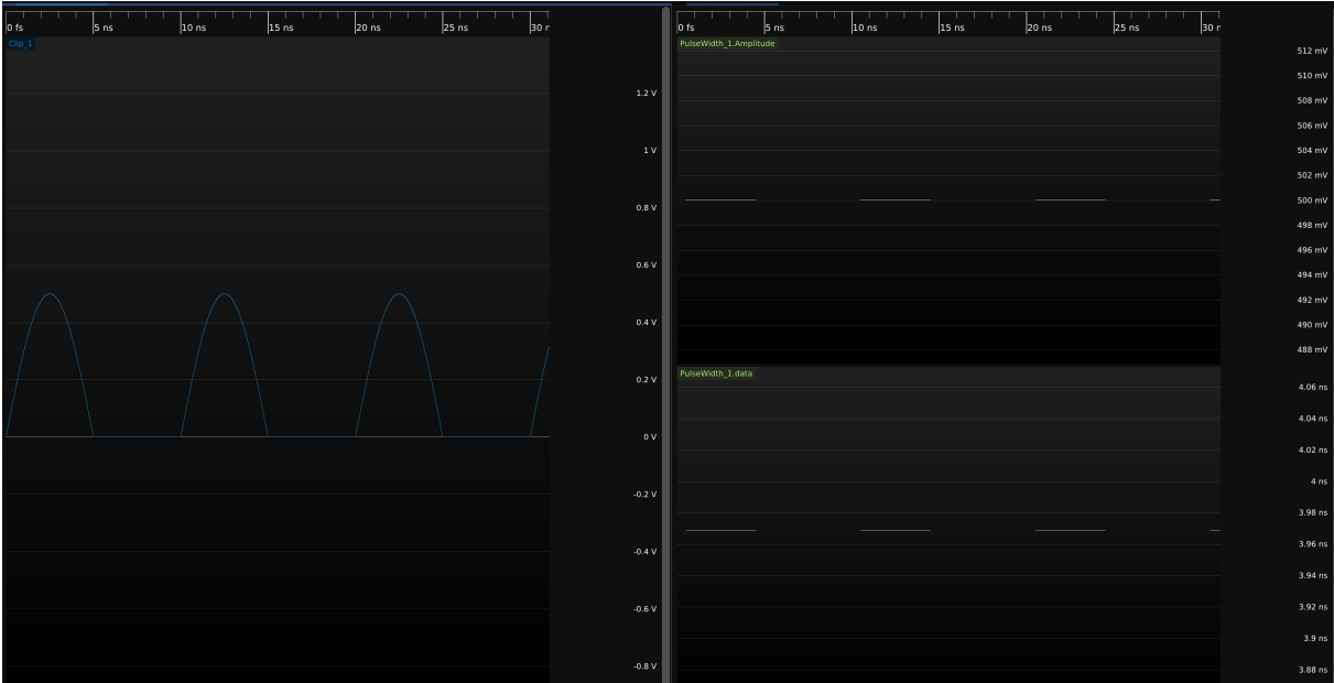
Figure 26.144: Example of pulse width measurement of a clipped sinewave input waveform.
