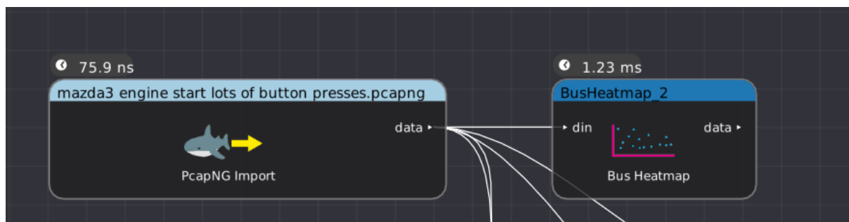
Figure 26.34: Example filter graph showing usage of bus heatmap filter on an imported CAN bus capture
