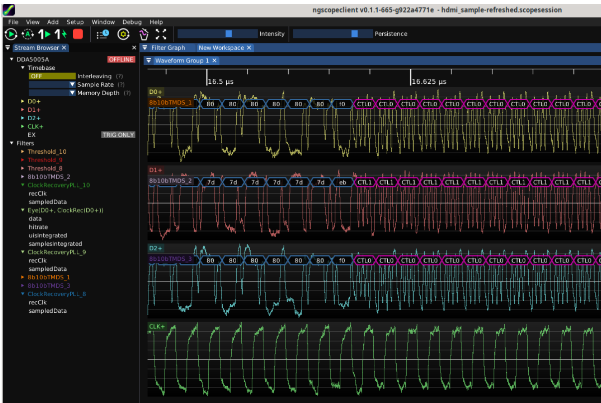
Figure 26.9: Example TMDS decode
