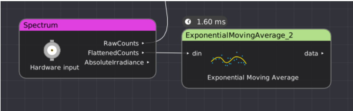
Figure 26.124: Example filter graph showing usage of exponential moving average filter
