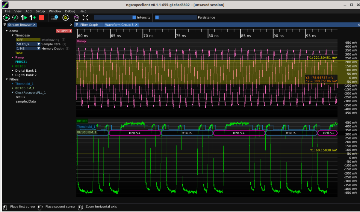
Figure 9.5: Single and double horizontal cursors
