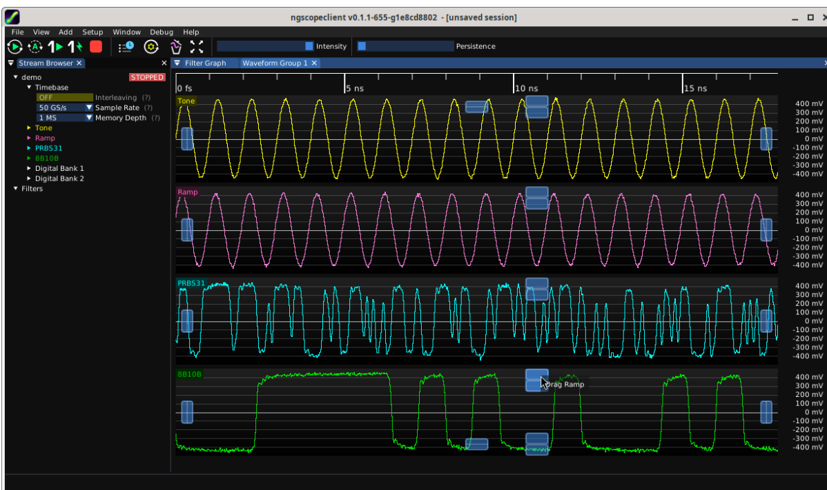
Figure 8.2: Overlays showing drag-and-drop locations for splitting waveform groups
