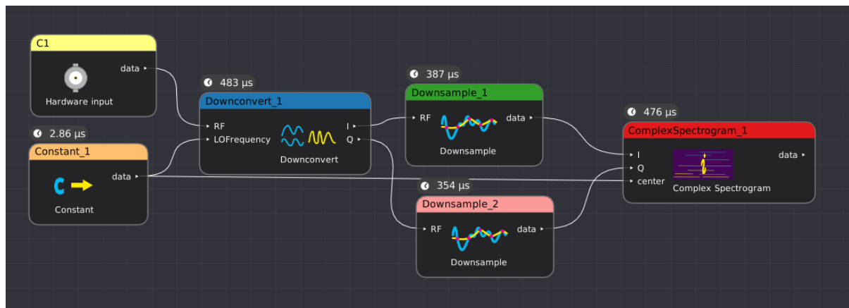
Figure 26.83: Example filter graph downconverting a 2.437 GHz Wi-Fi signal to zero IF, decimating and filtering, and displaying a spectrogram
