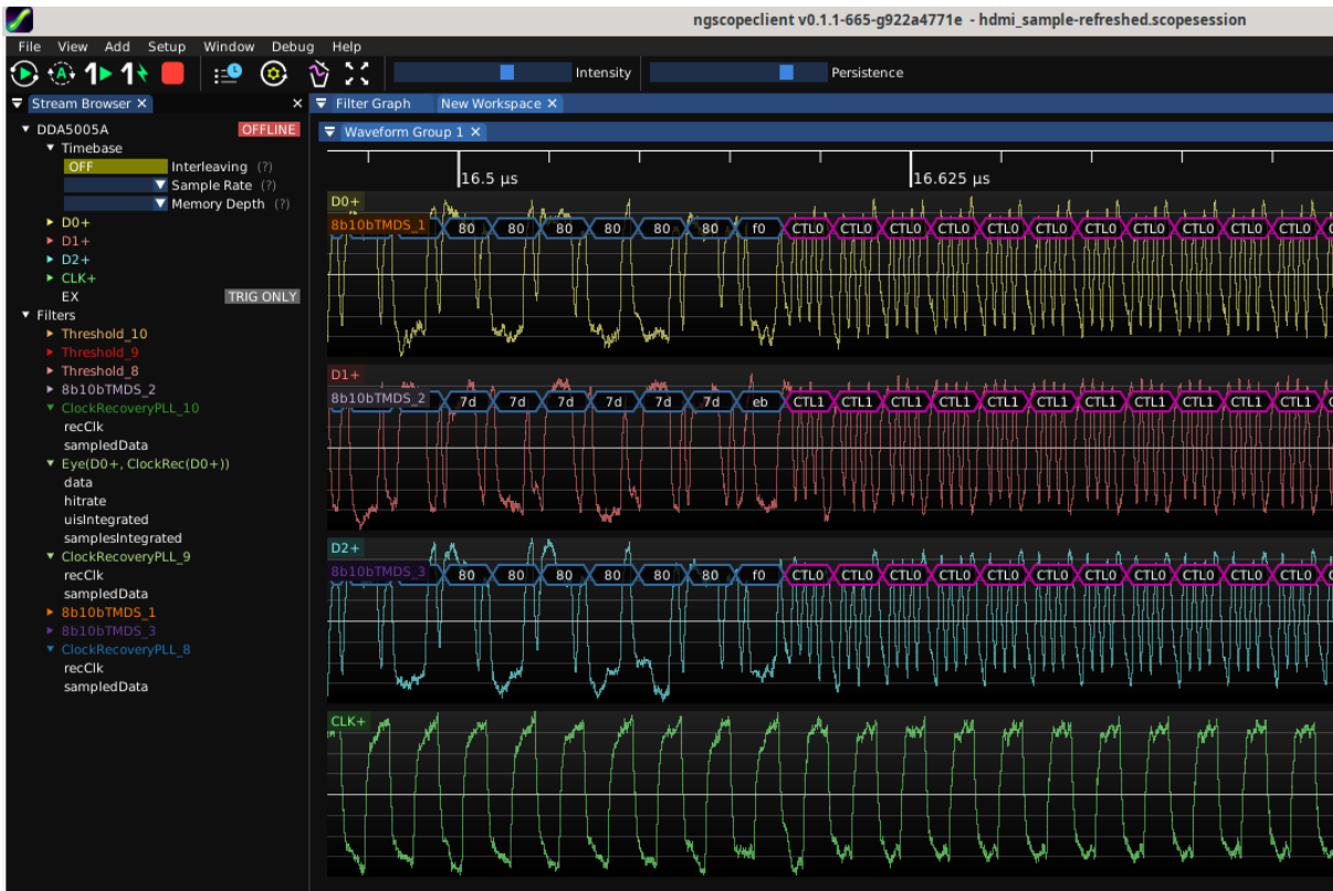
Figure 26.88: Example of decoding a DVI signal
