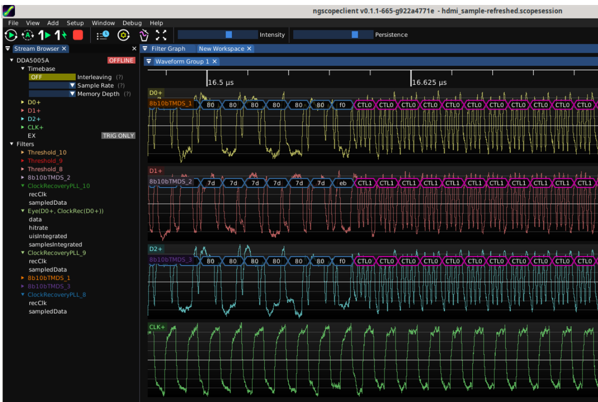
Figure 26.9: Example TMDS decode
