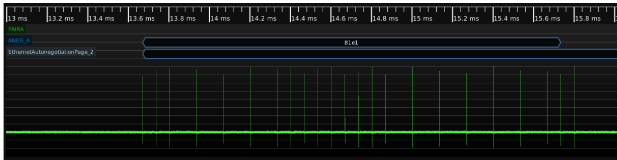
Figure 26.119: Decoding a single 16-bit link code word
