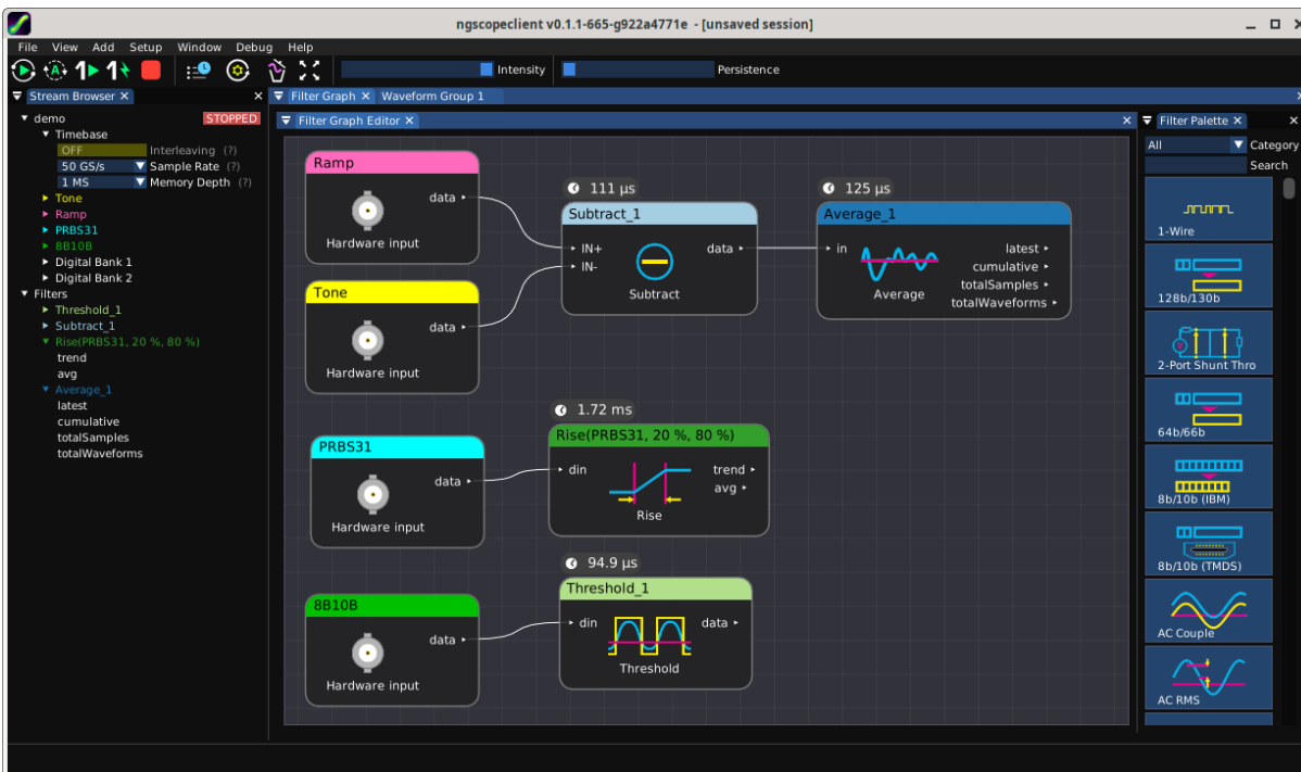
Figure 12.1: Filter graph editor showing instrument channels and several processing blocks
