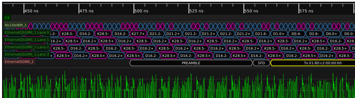
Figure 26.67: Example of decoding a QSGMII signal
