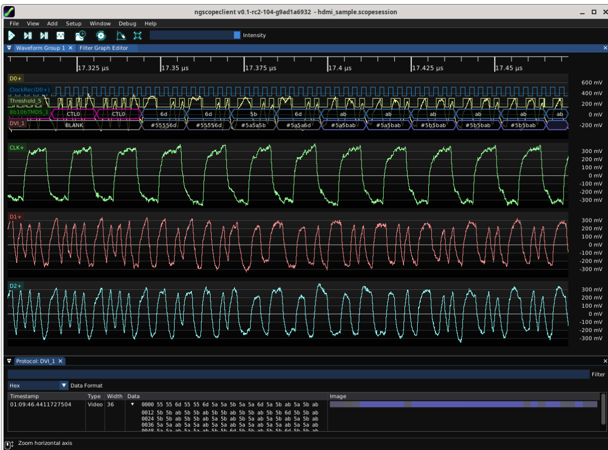
Figure 26.7: Example TMDS decode
