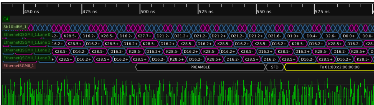
Figure 26.67: Example of decoding a QSGMII signal
