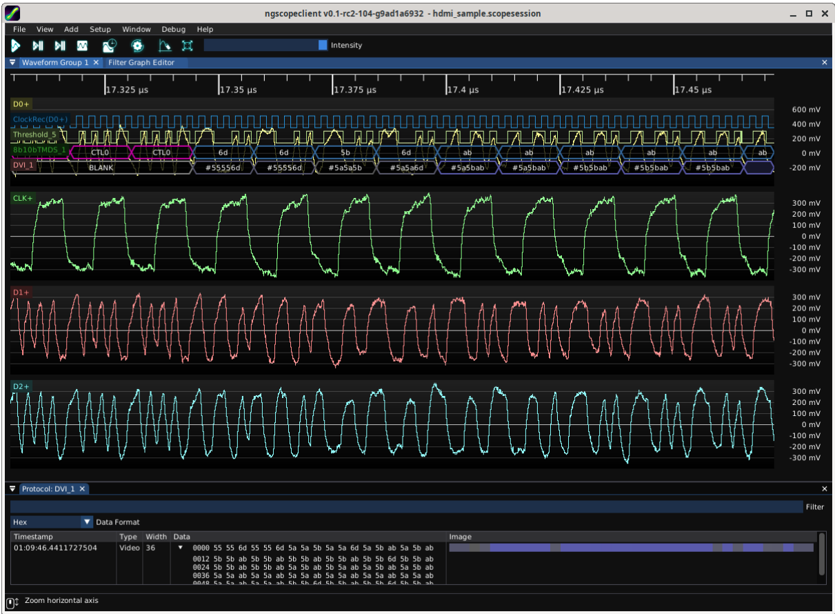
Figure 26.61: Example of decoding a DVI signal
