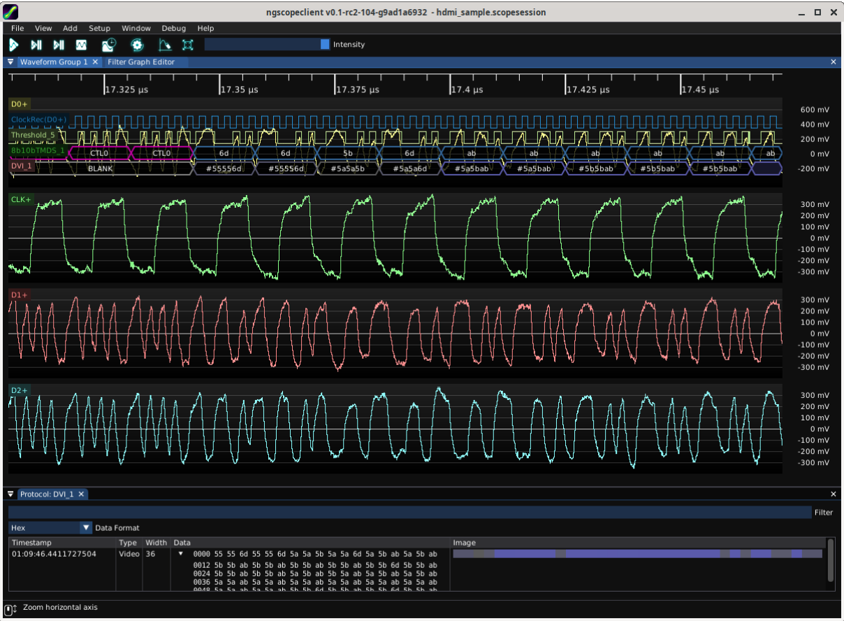
Figure 26.61: Example of decoding a DVI signal
