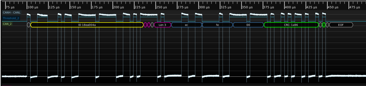
Figure 26.31: Example of decoding a single extended-format frame with 3 bytes of data
