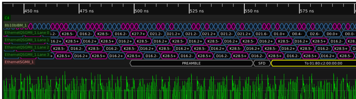
Figure 26.67: Example of decoding a QSGMII signal
