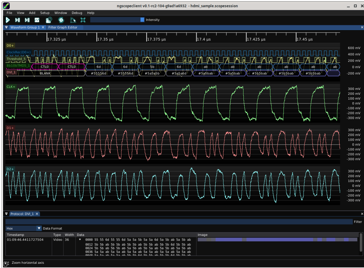
Figure 26.61: Example of decoding a DVI signal
