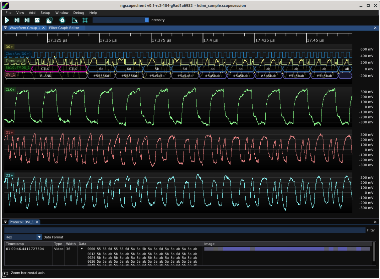
Figure 26.61: Example of decoding a DVI signal
