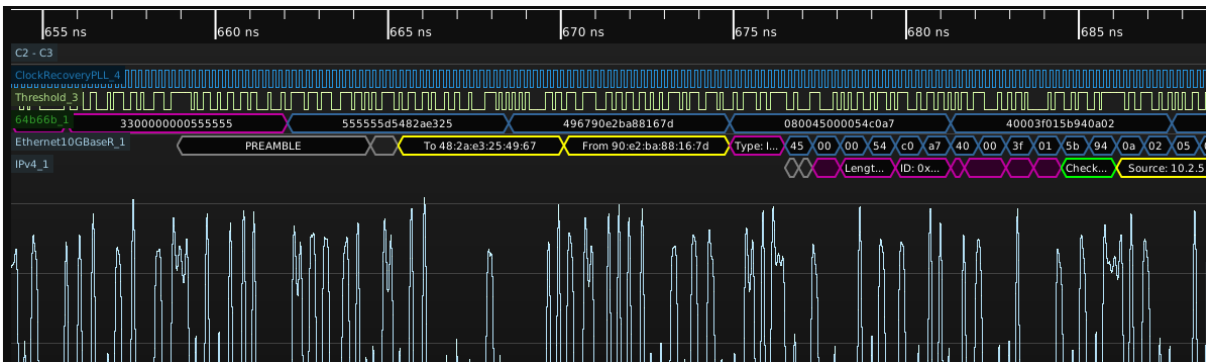
Figure 26.3: Example 64b/66b decode
