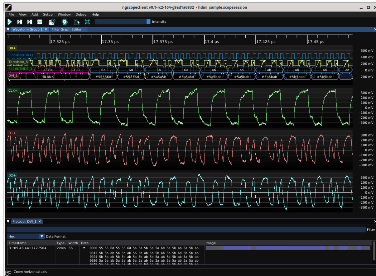
Figure 26.61: Example of decoding a DVI signal
