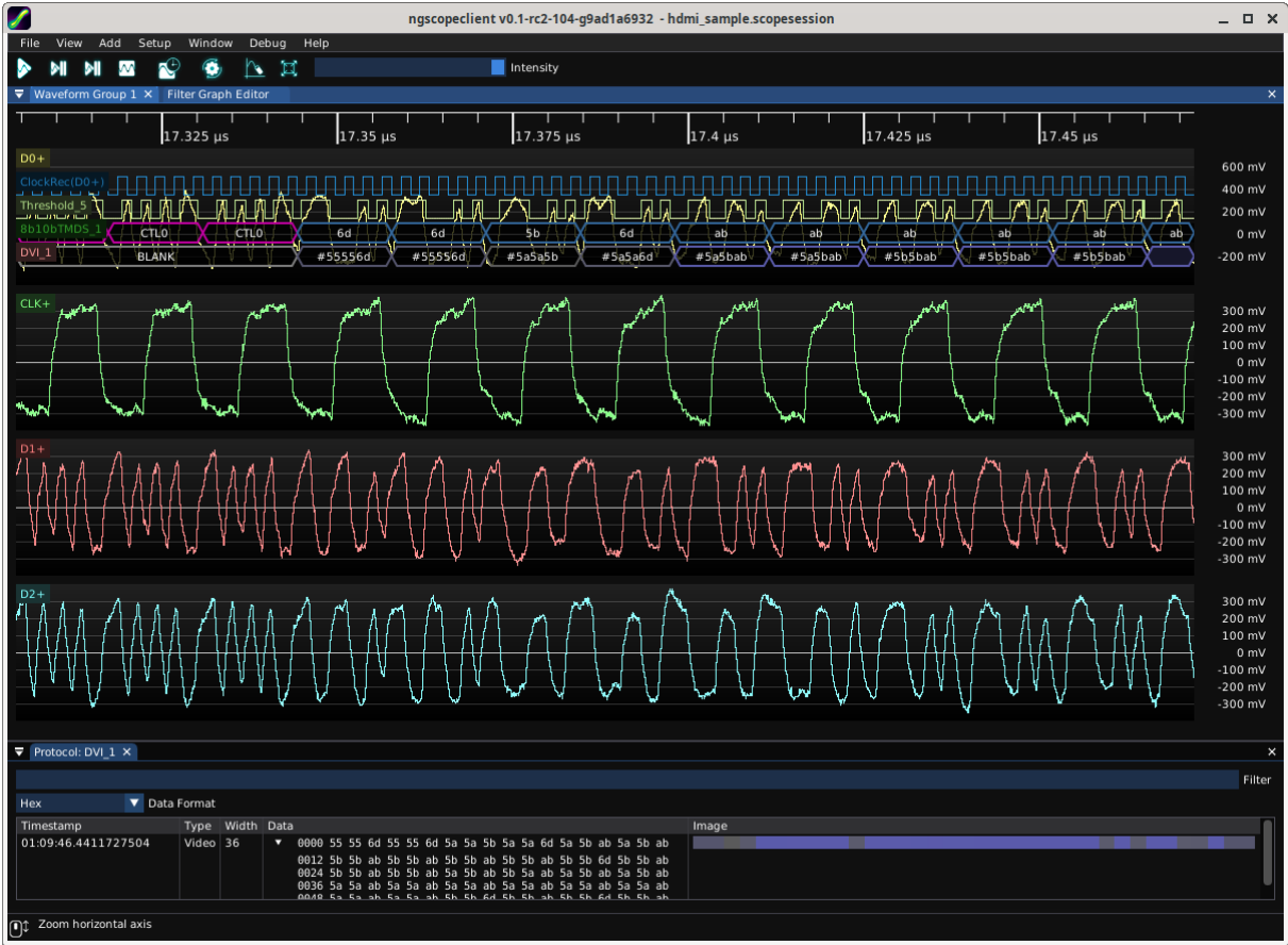
Figure 26.61: Example of decoding a DVI signal
