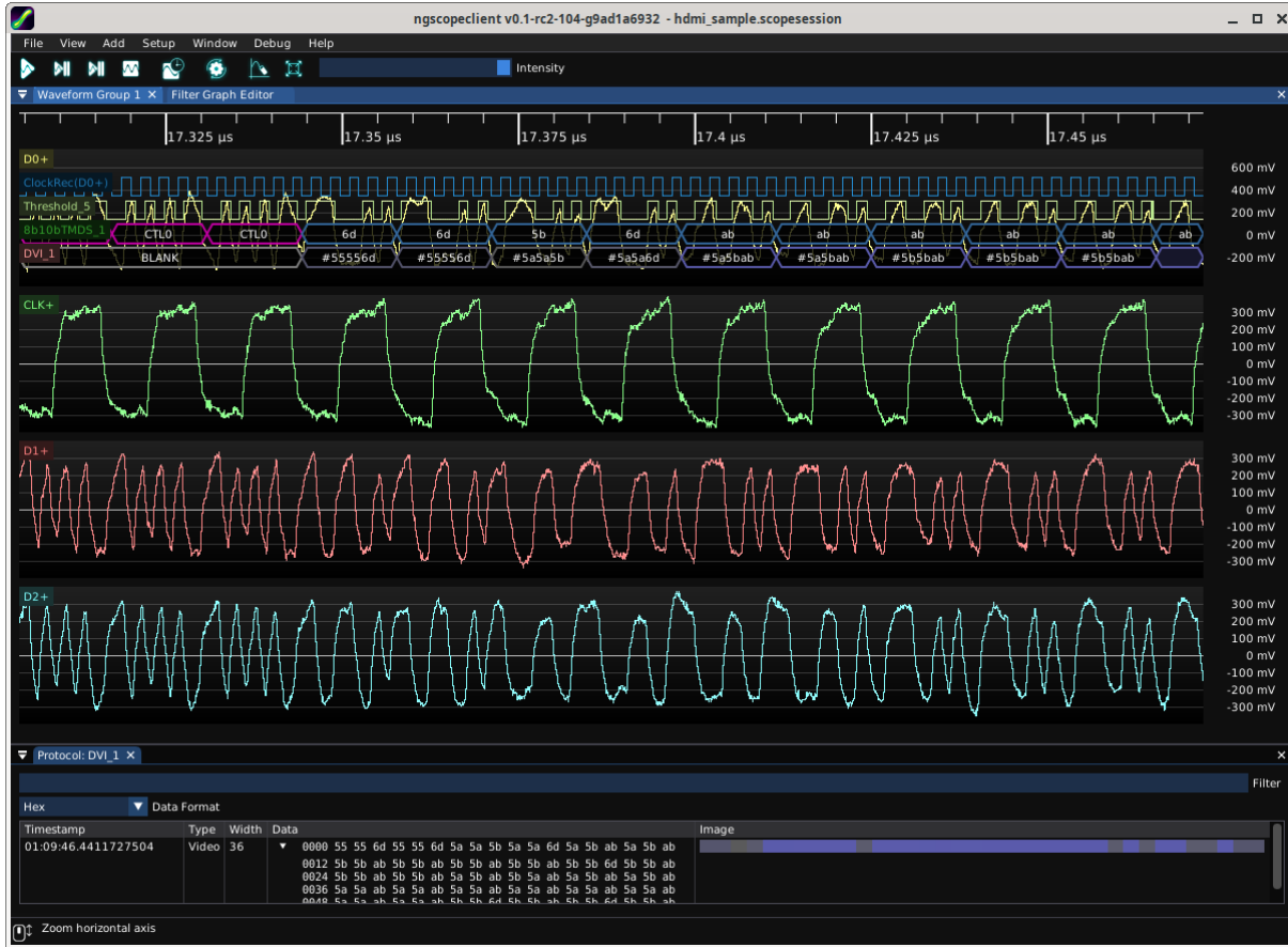
Figure 26.61: Example of decoding a DVI signal
