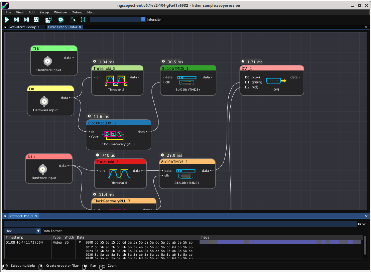
Figure 26.62: Example filter graph showing usage of DVI decode filter
