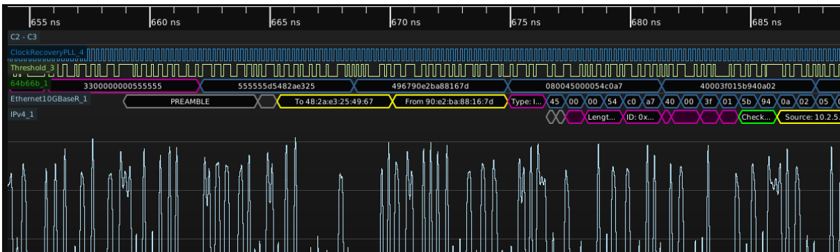
Figure 26.3: Example 64b/66b decode
