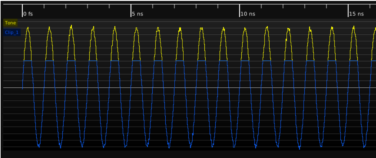
Figure 26.38: Example of clipping a sinewave
