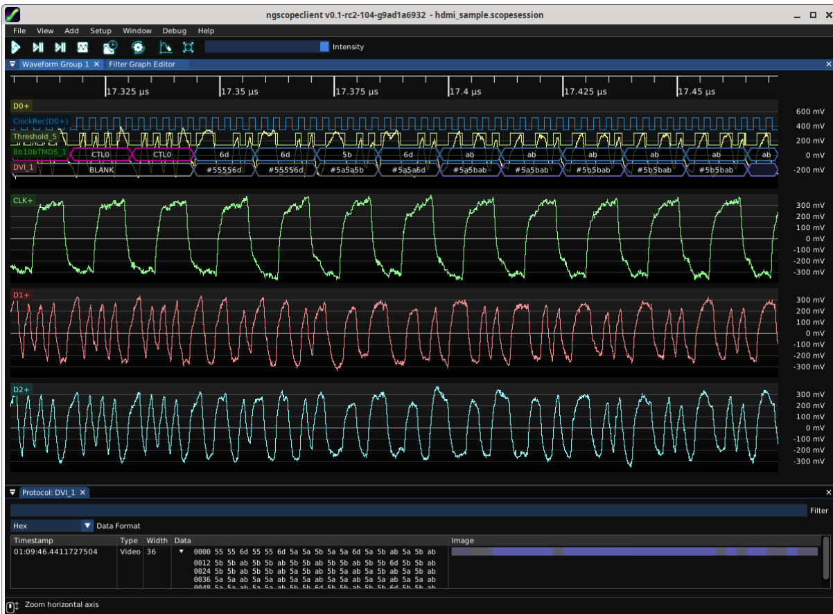
Figure 26.7: Example TMDS decode
