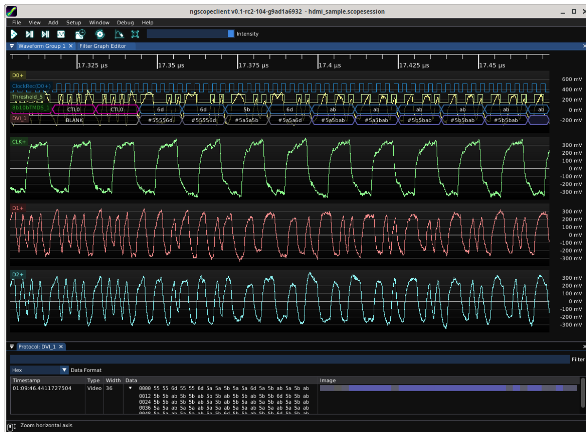
Figure 26.61: Example of decoding a DVI signal
