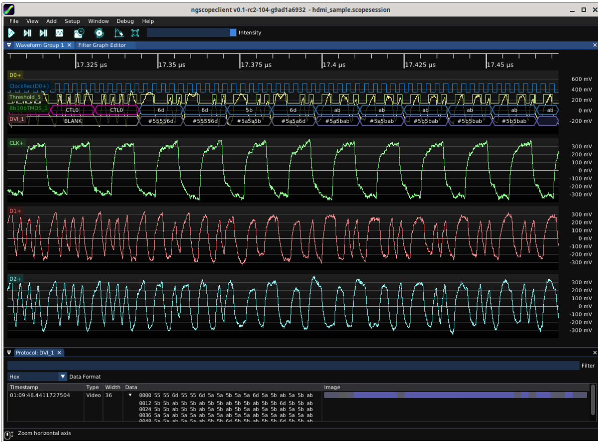
Figure 26.61: Example of decoding a DVI signal
