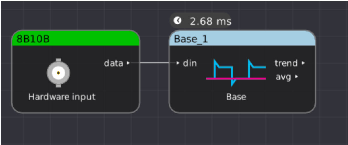
Figure 26.26: Example filter graph showing usage of base filter
