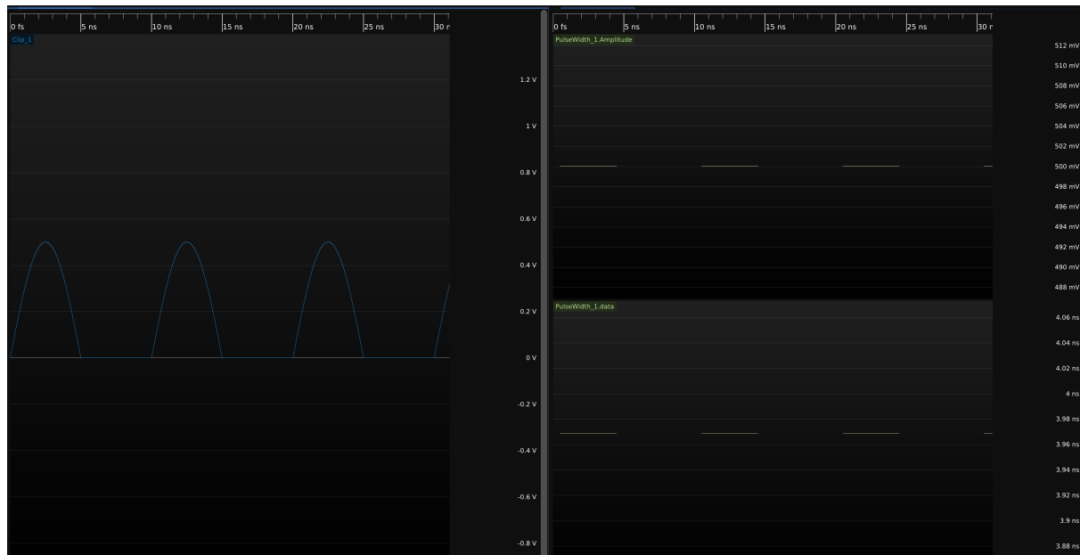
Figure 26.79: Example of pulse width measurement of a clipped sinewave input waveform.
