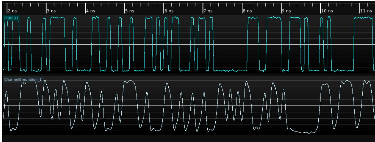
Figure 26.36: Example of channel emulation on a serial data stream
