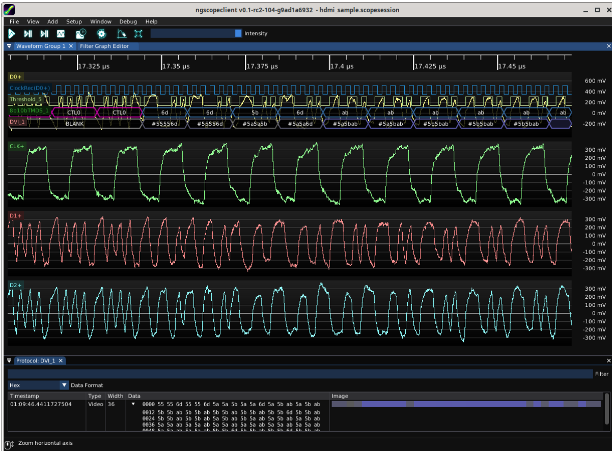
Figure 26.61: Example of decoding a DVI signal
