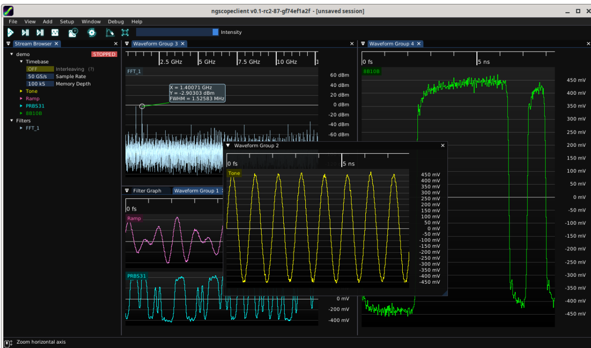
Figure 8.4: Example of complex window layout with multiple tabs, splitters between docked waveform groups, and a group in a floating window
