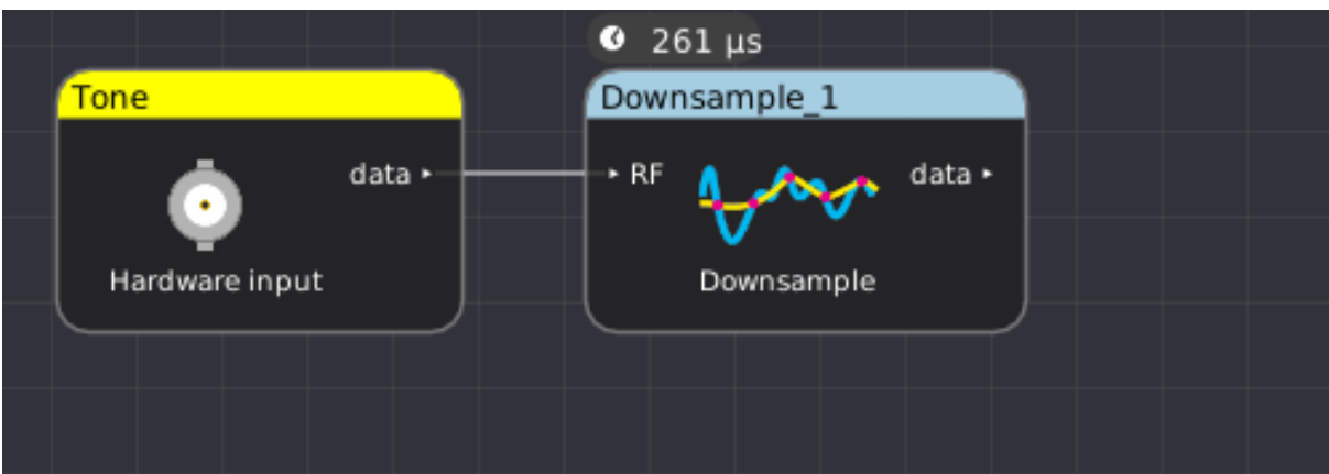
Figure 26.58: Example filter graph showing usage of downsample filter
