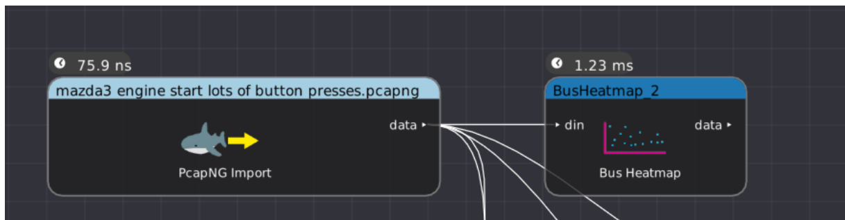
Figure 26.30: Example filter graph showing usage of bus heatmap filter on an imported CAN bus capture
