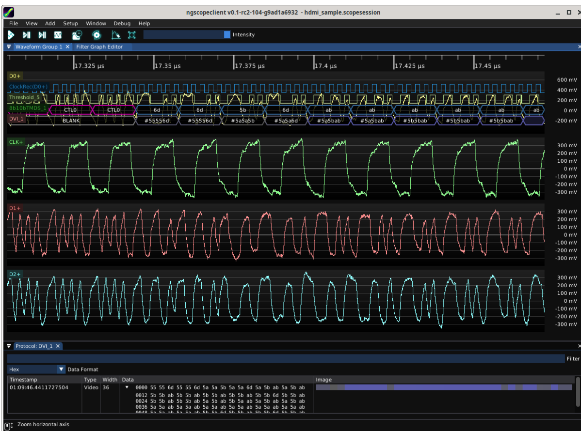
Figure 26.7: Example TMDS decode
